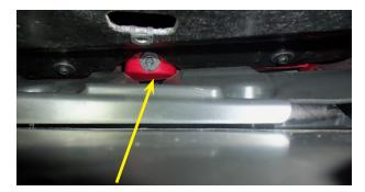
• With the chin spoiler removed, take out the rest of the belly pan bolts and remove the belly pan. After the system is installed reverse these steps to reinstall the belly pan and chin spoiler.
