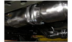
• Temporarily install the cats and x-pipe in order to mark the location where the factory exhaust needs to be cut for removal of the factory resonator and installation of the x-pipe extension tubes.
