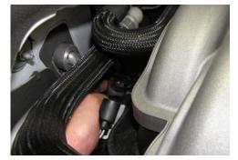
• While the vehicle is still on the ground, remove and unplug the front O2 sensors located between the rear of the engine and firewall above the transmission bell housing. Install left and right front O2 sensor extensions at this time.
