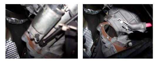
• Next lift the front of the engine up as far as it will go; the bell housing of the transmission will hit the firewall preventing you from lifting the engine too high.
