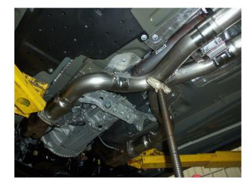
• Place wood wedges at the end up the x-pipe extension tubes as shown. Note the ends of the x-pipe extension tubes are angled to allow the tubes to be adjusted for proper clearance when rotated.
