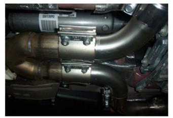
Next install the rear 02 sensor extensions into the factory wiring harness. Install the left and right 02 sensors into the convertors. Plug the extensions and 02 sensors together and use the supplied wire ties to tie up the wires away from coming into contact with any part of the exhaust. **End of Shelby mid-section installation go to the next steps on page 18.**
