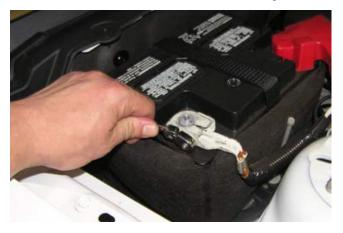
• Remove wiring harness from battery tray before removing the battery tray.
