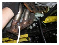
· Remove 02 sensors from manifolds.
