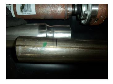
· Cut factory exhaust where marked and deburr tubes inside and out.
