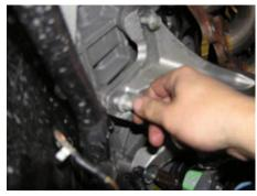
• Remove both the left and right engine mount.
