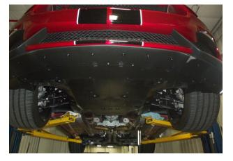
Next there are four screws holding the center of the chin spoiler that need to be removed. These can be accessed through the rectangular openings towards the front of the belly pan with an extension. The center chin spoiler must be removed to get the remaining belly pan bolts holding the front of it on. Photo showing one out of the four.
