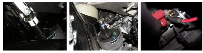
Remove the red plastic cap protecting the starter terminals and disconnect the wiring from the terminals.
