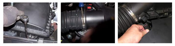
• Check all work for completeness, bolts tightened, connectors connected, and lines replaced and clamped etc. Check that no wires or lines are close to the headers where heat damage could occur or near moving parts where they could be pinched or cut. Check for misplaced tools and rags and check for oil leaks etc.
