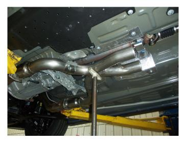
· Slide x-pipe extension tubes onto x-pipe and mark final cut location of the factory exhaust.
