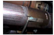
• Next remove the catalytic converters from the manifolds.
