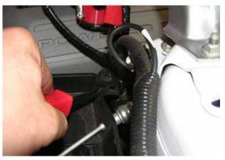
• Removal of the battery and tray provides more room to get to the manifold bolts during a later step. Remove the battery cover and tie-down, the battery, and finally remove the battery tray by removing the 3 bolts holding the tray in position.
